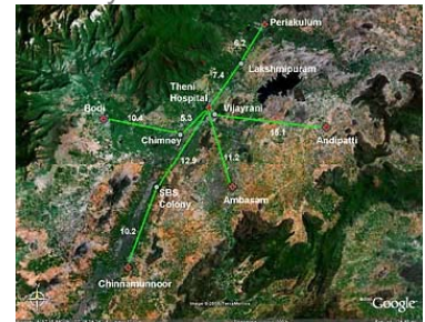
Map of wireless network connecting rural clinics to central hospital (map by Sonesh Surana)
